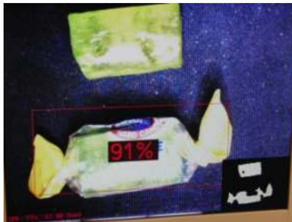
Example of an operator status display showing the ‘score’ of objects. The unwrapped candy does not meet all requirements to be scored, and will be rejected, whereas the wrapped candy has a score of 91% and will be accepted
